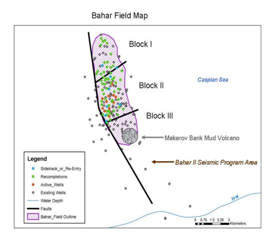
Gas and condensate distributed within the stratigraphic section indicate that these multi-bedded gas and condensate accumulations occur within a single hydrodynamic system. Gas accumulations contain a significant amount of condensate, which increase in richness with depth. Reservoir rocks (sandstone and siltstones) are of good quality. Average porosity ranges from 14 to 22% and average permeability ranges from 12 to 166 md. Water saturation in the pay intervals ranges from 8 to 56%.
